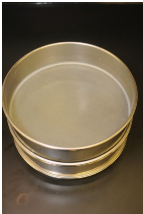
Figure 17.1 Mesh sieve used to determine particle size when compounding dry powders for topical use.
